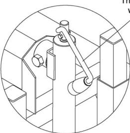
This illustration shows the position where the handle be when the disc is in use.
