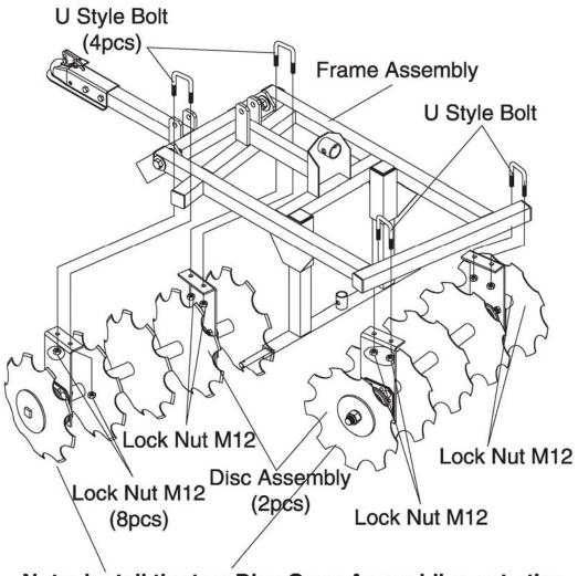
Note: Install the two Disc Gang Assemblies onto the frame in the opposite direction.
