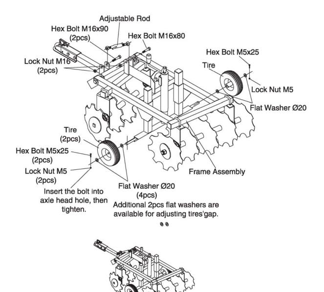
Step 6: There maybe some adjusting of the Hitch Tongue for the height of towing vehicle, this function can be performed by rotating handle on Adjusting Rod. Rotating the handle on the Mechanical Screw Jack will raise the tires up down.
