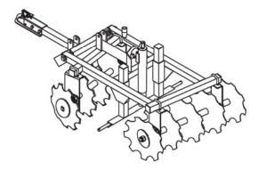
Step 5: Install Adjustable Rod to the Hitch Tongue and the Frame using the Hex Bolts and Lock Nuts as Shown. Install the Tires onto the Wheel bracket using the Flat Washers, Hex Bolts and Lock Nuts as shown.
