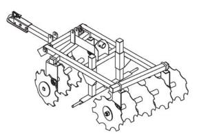
Step 4: Install the Mechanical Screw Jack onto the frame as shown in the diagram using the Hex bolts and Lock Nuts.
